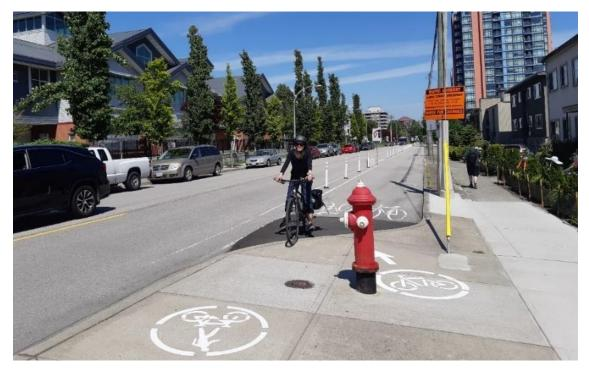
Example of a quick-build cycling facility on Agnes street (New Westminster, BC). A similar facility is recommended on Esquimalt Road as part of the quick-build network.
