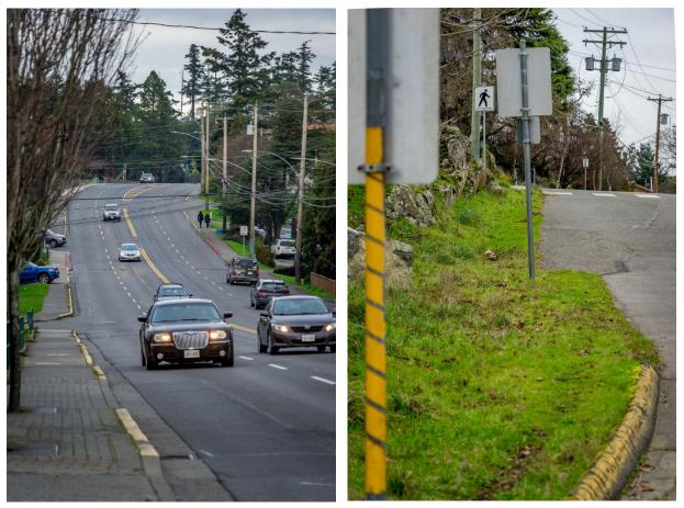
Tillicum Road (left) emerged as an area of concern for pedestrians in the public engagement citing the lack of separation between the sidewalk and motor vehicle travel lane and challenges crossing the road. Segments along Lyall Street (right) have discontinuous sidewalks. In this photo, a person using a mobility device (e.g., walker, wheelchair) would have challenges access the crosswalk.
